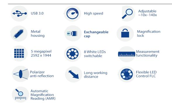
The Dino-Lite AM73515MZTL is a USB 3.0 model with a magnification range of 10x - 140x and a Long Working Distance of up to 24 cm. This model is member of the Dino-Lite Edge family with the latest, cutting-edge optics, an unmatched 5 megapixel sensor and several special features such as:
