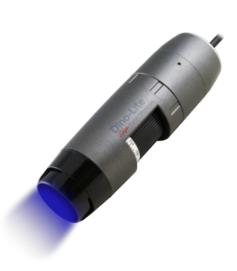
Short Description1.3 Megapixel resolution480nm excitation and 510nm emission filter20-220x magnificationTo observe GFP, FITC
